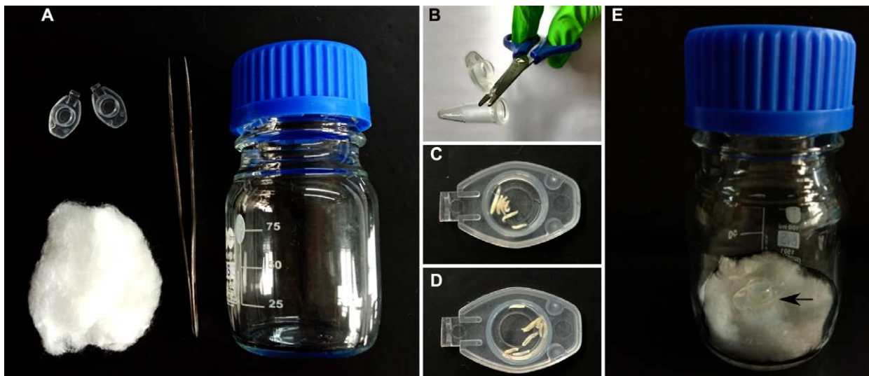
Fig. 1. Setup for immobilizing larvae by ether anesthesia. A. Components of the setup for larval anesthesia. B. Cutting off the cap of 1.5 mL microfuge tube with scissors. C. Larvae in PBS in the space in microfuge tube cap. D. Larvae in the cap after aspirating out of the PBS. E. Larvae in the cap (arrow) being exposed to ether in the closed bottle with ether-soaked cotton.
