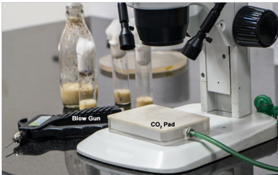
Fig. II. 2. Commercial CO 2 Fly pad placed at the base of a stereobinocular microscope enables viewing the immobilized flies.
