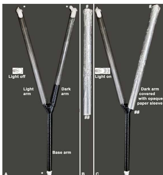
Fig. 1. The Y-maze for phototaxis assay. A. Y-maze glass tube with black tape tightly wrapped around the base arm; * = cotton plugs covering three open ends of Y-maze. B. Opaque paper cylindrical sleeve with one close (#) and one open end(##). C. Y-maze with one arm (dark arm) covered with the opaque paper sleeve.
